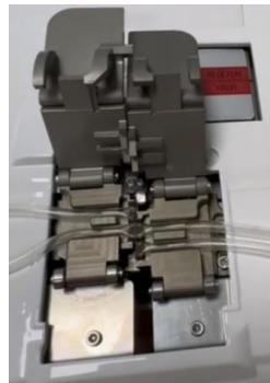
3. After the joining is completed, open the catheter pressure plate and take out the catheter.
