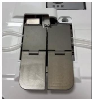
1. Install the pipeline properly, fasten the pipeline pressure plate tightly, and press the start button.
